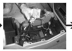
**STEP 9:** Once the wire harness is unsecured, disconnect the white plug.
